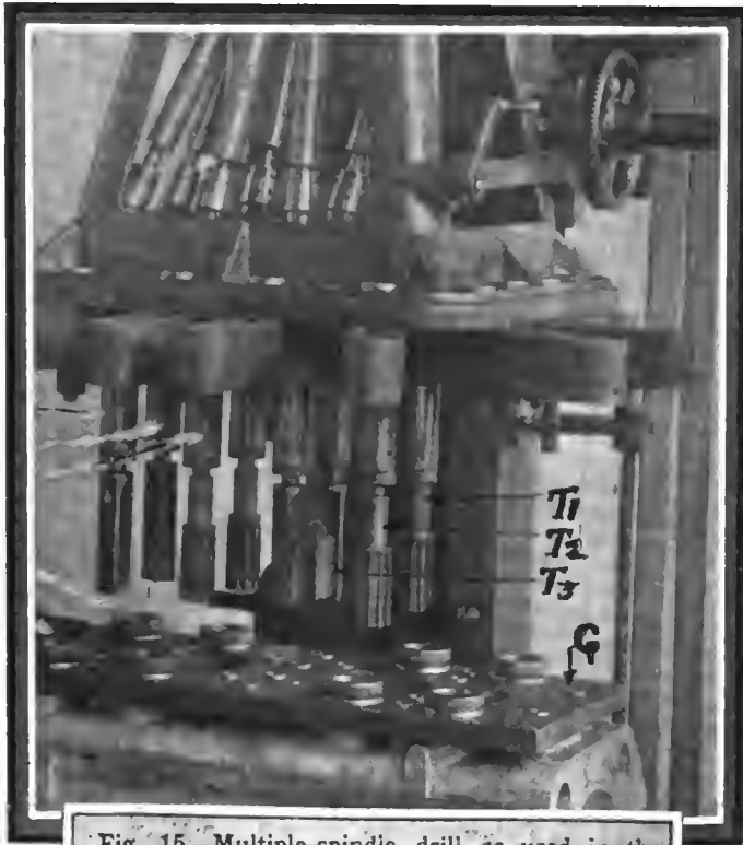
Fig. 15—Multiple-spindle drill as used in the Marmon plant in conjunction with a jig for crankcase work
